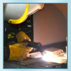
The American Welding Society Handbook, 9<sup>th</sup> Edition Volume 2 on page 666 presents cost data comparing Plasma Gouging and Air Carbon Arc Gouging. They show for a specific gouge, the cost for Plasma Gouging is \$0.16 per foot of gouge while Air Carbon Arc Gouging cost \$0.42/foot.
