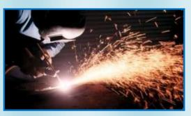
Welding fumes, as noted above, may be over 10 times lower with Plasma Gouging. However when gouging carbon steel, fume measurements must still be made with Manganese being the element that will probably be the deciding factor to define adequate ventilation to protect the operator. For stainless steel, Chrome VI will usually be the element requiring measurement and control. Gases, such as Ozone, could also be an issue depending on venation conditions.
