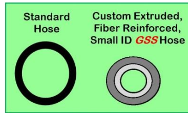
GSS hose volume 75% less than 1/4 hose
